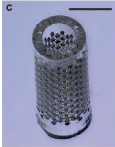
Micro filter element with 55 \mu\text{m} holes
